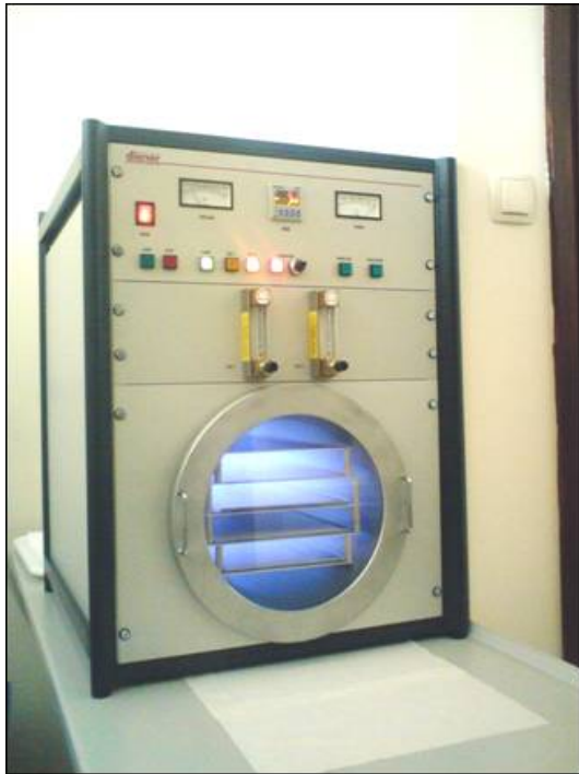
Low-pressure plasma system typ NANO, LF-40kHz, by Diener Electronic
