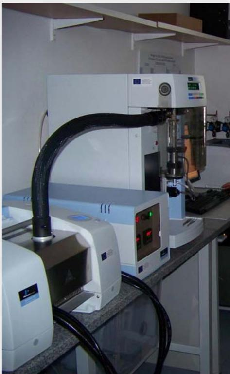
Thermal analyses of cotton materials were performed in a flowing synthetic air atmosphere (30 % oxygen; flow rate of 90 ml/min) using a Perkin Elmer analyzer controlled by a PC system. TG (thermal gravimetric) of the samples were obtained from 20 to 800 °c in air at a heating rate of 30 °c/min. prior to the thermal analysis runs the cotton fabrics were cut into small pieces having an average weight of ca. 1 mg, whereas the analyzed samples weighed approximately 6 mg.
